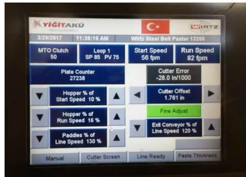
HMI control of three (3) Variable Speed Drive(s) ensures optimum paste delivery, flow and fill, for all paste 'variants' (oxide, density, moisture, rheology 'flow' and additives).
