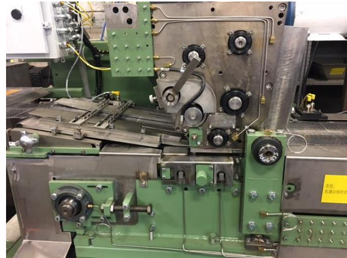
**Patented SERVO control adjusts the pasted plate thickness 'on the fly' in 0.0005 inch (.0127mm) increments, controlled from a 'high precision', dynamic (in motion) closed-loop plate weight or thickness monitoring device.**
