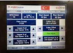
HMI control of three (3) Variable Speed Drive(s) ensures optimum paste delivery, flow and fill, for all paste 'variants' (oxide, density, moisture, rheology 'flow' and additives).
