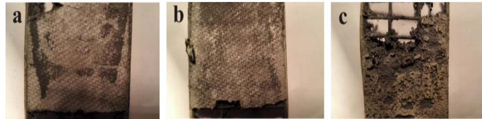
Digital pictures of Control, RHC and KAC after PSoC test.
